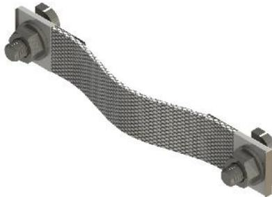
The Fast-Rack Bonding Jumper Kit is used to electrically bond adjacent rails together when necessary. Each kit includes bonding strap, 2 bonding plates and 2 T-Bolts with flange nuts.
